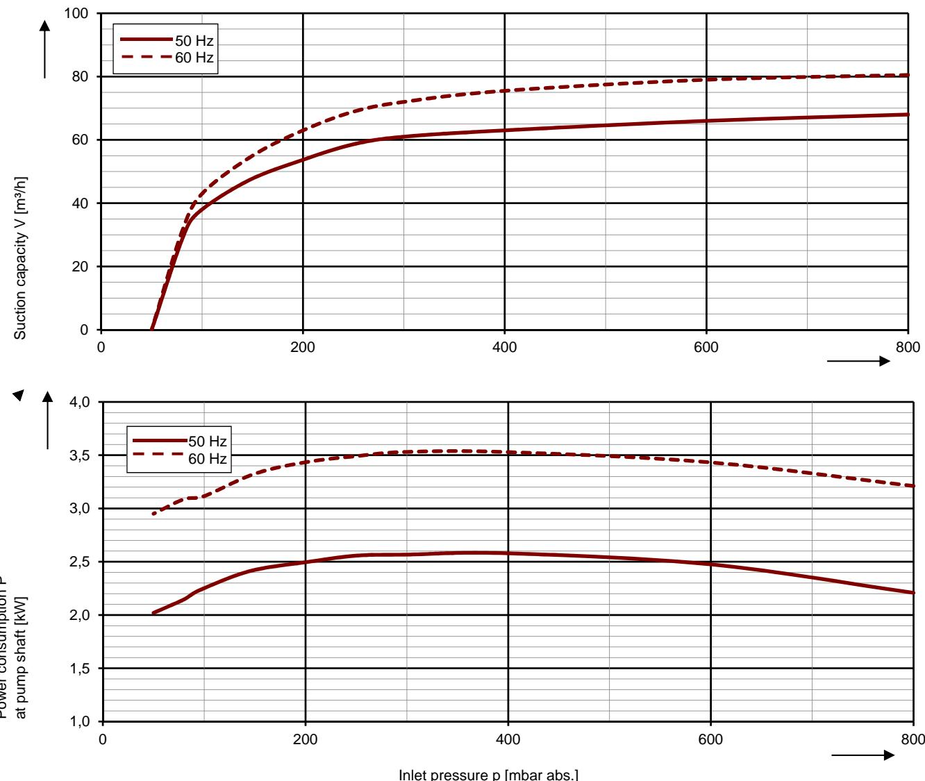
The characteristic curves are based on the evacuation of dry air and an intake temperature of 20 °C. At a suction pressure of 1013 mbar abs. (water as operating liquid) the characteristic curves will be achieved. The tolerance is ± 10 %.
