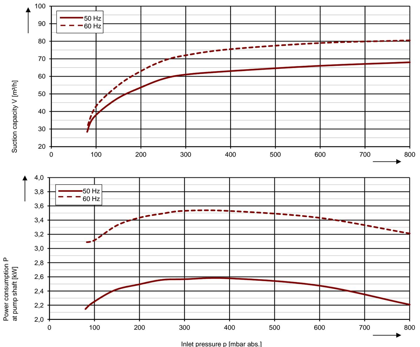
The characteristic curves are based on the evacuation of dry air and an intake temperature of 20 °C. At a suction pressure of 1013 mbar abs. (w ater as operating liquid) the characteristic curves will be achieved. The tolerance is ± 10 %.
