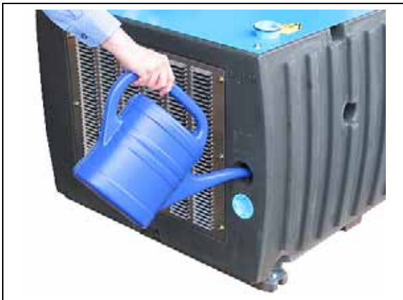
Fig. 8: Filling separator Models 2BL2 251 - 341 (via the filling opening)
