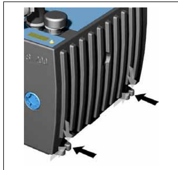
Fig. 4: Points for measuring the vibration speed
