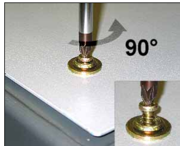
Fig. 5: Remove cover plate: Unscrew screws
