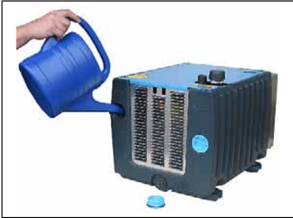
Fig. 7: Filling separator Models 2BL2 041 - 141 (via the filling opening)
