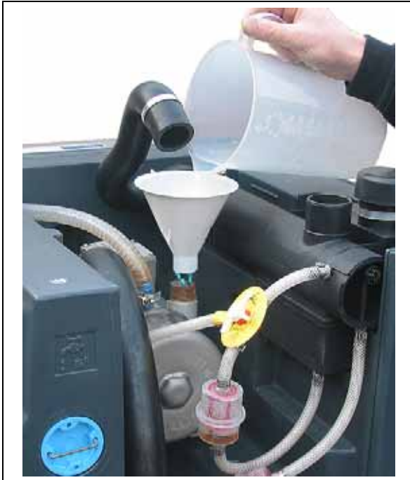
Fig. 13: Pouring anti-corrosive agent into installed unit (for models 2BL2 041 - 2BL2 141)
