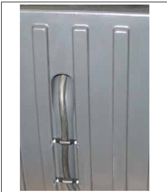
Fig. 6: Strain relief: Cord grips on the outside of the separator
