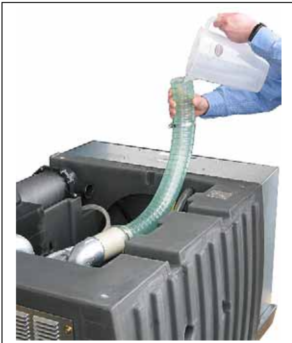
Fig. 14: Pouring anti-corrosive agent into installed unit (for models 2BL2 251 - 2BL2 341)
